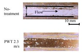
Fig. 5 Photographs of scaled heat transfer surfaces for Notreatment and PWT cases. Both 2,000  $\mu S/cm$
