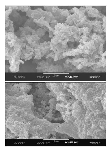
Fig. 6 SEM (scanning electron microscopy) photographs: top = no treatment case, bottom = PWT-2.3 m/s case, both 2,000 S/cm
