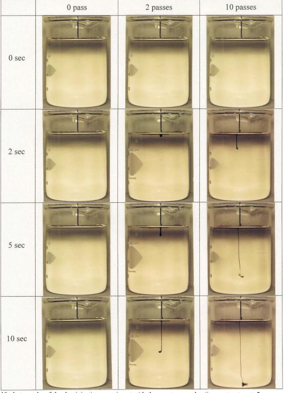
Fig. 10 photographs of the dye-injection experiment with three water samples (i.e., no-treatment, 2 passes, and 10 passes through the solenoid coil). Water conductivity =  $3,000 \mu S/cm$
