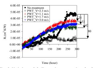
Fig. 3 Variations of fouling resistance vs. time for four different flow velocity cases through PMSM-1
