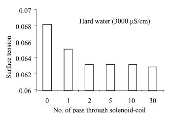
Fig. 9 The results of the surface tension of the sample water treated by a PWT (using a solenoid coil). Water conductivity =  $3,000 \mu \text{S/cm}$
